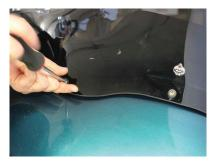
3. Starting with the center screw, install your new Flare™ Windshield and torque to factory specifications.
