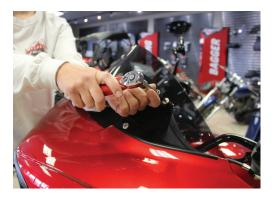
Carefully install the hardware removed in step 1 and torque them evenly to 50-60 in-lbs
