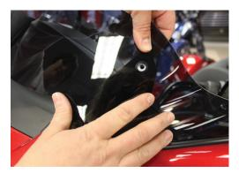
1. Using a 4mm Allen wrench, remove the four fasteners that hold the stock windshield to the mount brackets.
