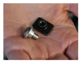
You can place low-tack tape on the back of the square nuts and bracket to help prevent them from falling into the fairing.
