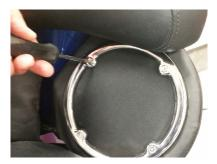
1. Remove the 4 fasteners that hold the speaker trim ring onto the rear speaker pod
